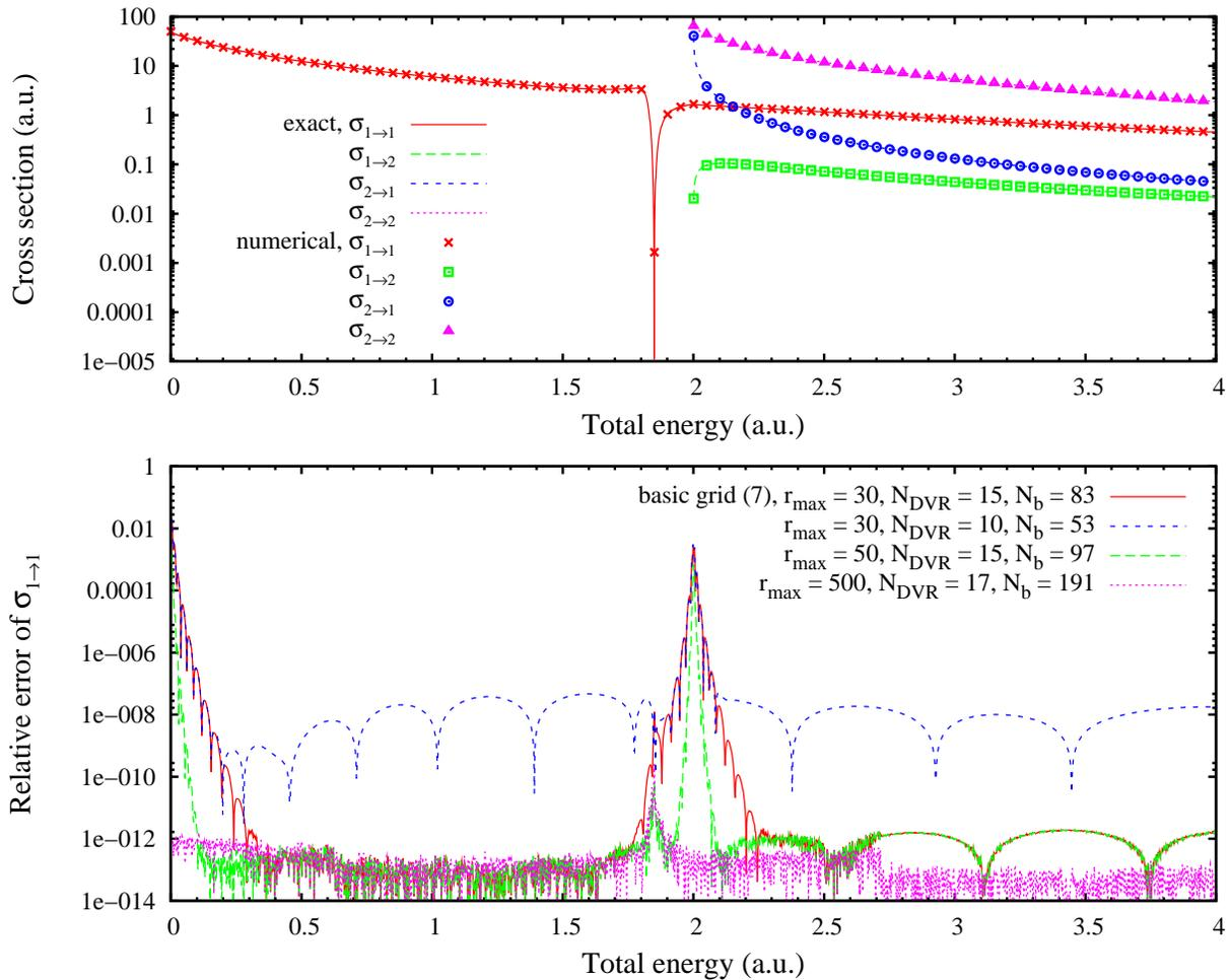
**FIGURE 2.** Upper panel: dependence of the cross sections for all transitions on the total energy (lines – exact results, points – numerical results). Lower panel: the relative error of the numerical values of the cross section  $\sigma_{1 \rightarrow 1}$  for four different grids.
