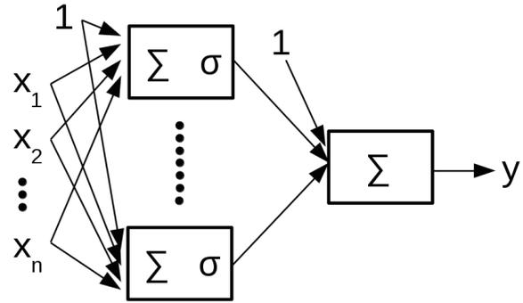
Fig. 1 Artificial neural network in the feed-forward configuration with a single hidden layer and scalar output  $y$ . Each synaptic connection denoted by an arrow has an associated weight parameter. Input aggregation is denoted with the symbol  $\Sigma$  whereas  $\sigma$  stands for the nonlinear activation function. The bias value for each neuron is represented by the constant input 1.
