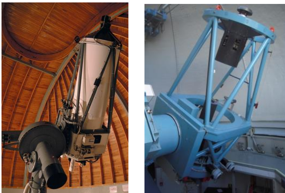
Figure 1: The 65-cm Charles University reflecting telescope at Ondřejov Observatory was built in 1972 by late Dr. Pavel Mayer (left, current photo by Kamil Hornoch). The Danish national telescope DK154 is located at La Silla observatory in Chile (right). Both telescopes are equipped with a CCD camera with a set of photometric filters and enable remote access.
