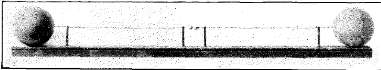
Figure 3—The First Oscillator of Hertz. Two copper wires, each 1 metre in length, supported on rods of sealing wax. The large spheres are of sheet zinc, and are 30 centimetres in diameter. Base 260 x 7.5 centimetres
