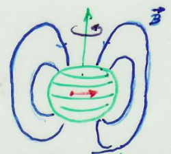
Rotating charged sphere \rightsquigarrow el. current \rightsquigarrow magn. field \vec{B}
