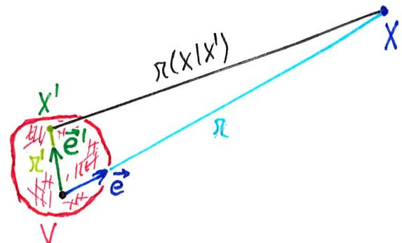
$$\vec{A}(x) = \frac{\mu_0}{4\pi} \underbrace{\frac{1}{r} \int_V \vec{j}(x') dV'}_{\text{monopol}} + \frac{\mu_0}{4\pi} \underbrace{\vec{r} \cdot \vec{e} \cdot \vec{e}'}_{\text{dipol}} \int_V \vec{r}' \vec{j}(x') dV' + \dots$$
