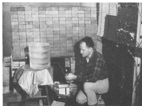
FIG. 3. In this scene taken from the film, Dr. Smith is shown assembling the detector. The iron shielding is in the background, and some of the electronics used can be seen on the right.
