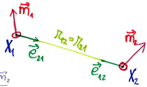
$$\vec{F}_{\text{mag1od2}} = \vec{\nabla}(\vec{B}_2 \cdot \vec{m}_1) = \frac{\mu_0}{4\pi} \vec{\nabla} \frac{3\vec{m}_1 \cdot \vec{e}_{12} \vec{e}_{12} \cdot \vec{m}_2 - \vec{m}_1 \cdot \vec{m}_2}{R_{12}^3}$$
