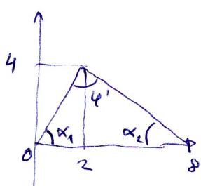
$$\left. \begin{aligned} \tan \alpha_1 &= \frac{4}{2} = 2 \Rightarrow \alpha_1 \doteq 63.43^\circ \\ \tan \alpha_2 &= \frac{4}{6} = \frac{2}{3} \Rightarrow \alpha_2 \doteq 33.7^\circ \end{aligned} \right\} \Rightarrow \varphi' = 1,447^\circ \quad \begin{matrix} \checkmark \\ \text{rounding error} \end{matrix}$$
